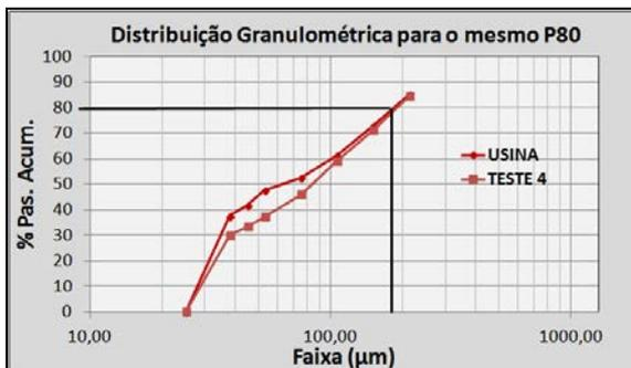
Figure 4.3 – Comparative Size Distribution of different grinding methods for the same P80
