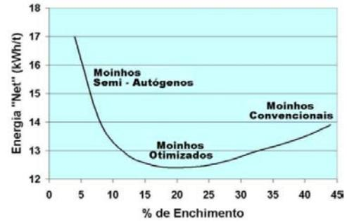
**Figure 4.1** – Filling level (Modelo Operacional)
