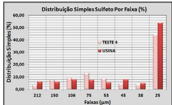
Figure 4.4 – Comparative Granulochemical Distribution of different grinding methods for the same P80
